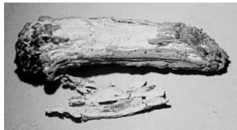
Fig. 2 Photography of a monolith of chitosan-templated siliceous material (CTSM). Length about 4 cm
